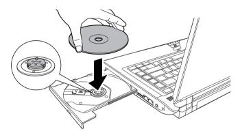
Inserting a disc
